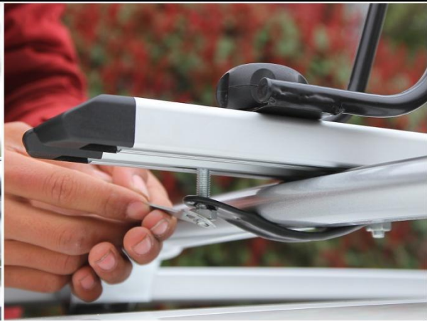
6. fix the rear aluminum spine by steel bracket
