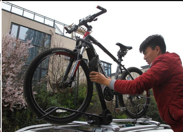
10. adjust the grip arm and secure the bike
