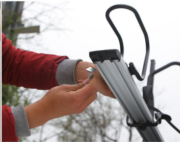
2. slide 2 T-bolts into the channels under the aluminum spine
