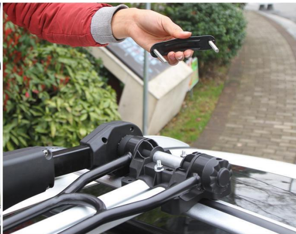
4. place the head unit on the front cross bar and fix
