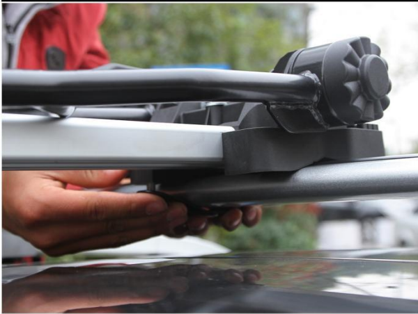
5. fix the head unit by steel bracket
