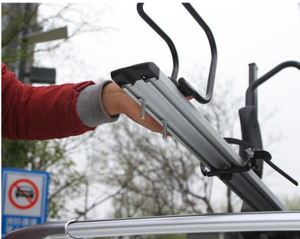
3. place the rear aluminum spine on the rear cross bar and fix
